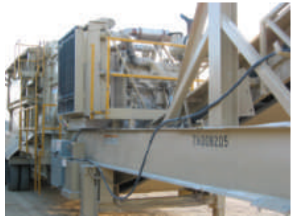
QSK19 Cummins Power Unit powering a gravel crusher.
